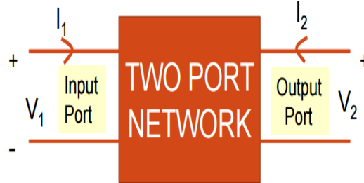
Fig 11: Two Port Network
