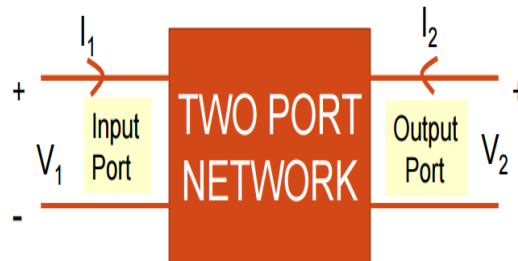
Fig 2. Two port Network
