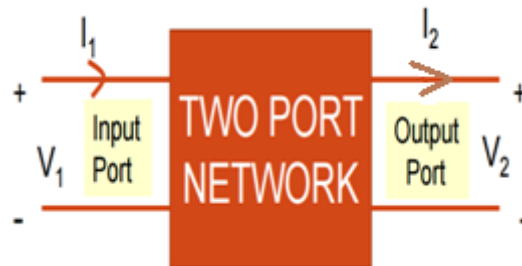
Fig 13: Two Port Network
