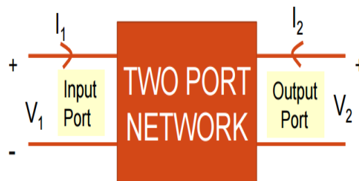
Fig 3. Two port Network
