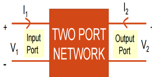
Fig 7. Two port Network
